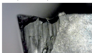
Tool wear after 39 minutes of machining
